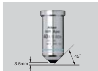
All objectives have wide approach angles and long working distances (45° and 3.5mm with 40x objective).
